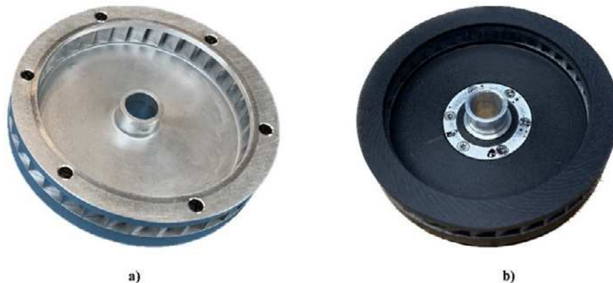
Figure 3: Comparison of: a) milled aluminum wheel ( Version 2 a, 2b and 2c ) and b) 3D printed plastic wheel ( Version 3 )
